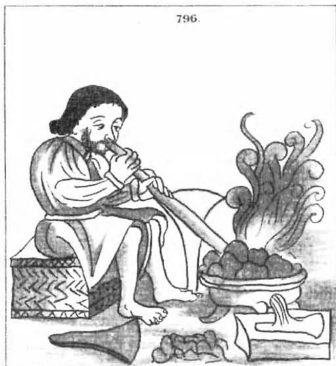
Figure 9. Metalsmith depicted in the Florentine Codex, Folio 796. Note the open mold of an axe into which it appears molten metal is flowing. Also note the brazier, possibly ceramic, into which the metal-smith is forcing oxygen through a hollow tube tipped with a tuyere (blowpipe tip).
