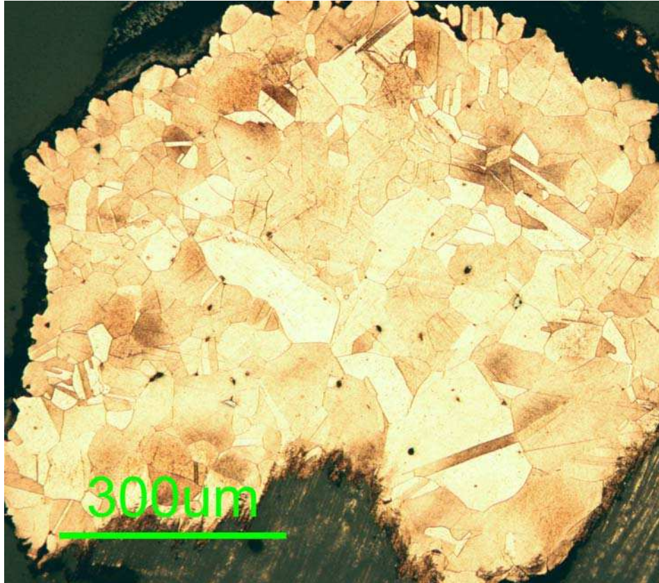
Figure 8: Bell LA 1238/1: Section at down sprue showing annealing twins and some deformed twins at the edges of the sample which could have resulted from cutting the sample.
