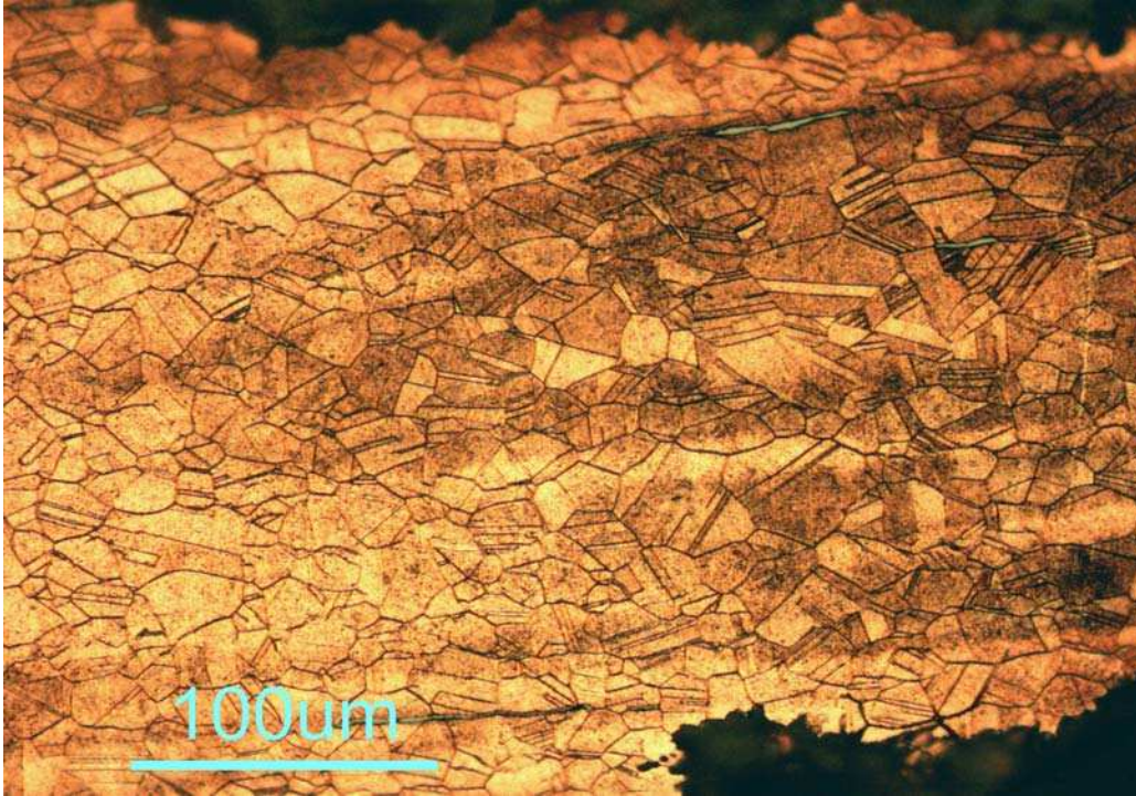
Figure 24: LA 1241/1: image showing the equiaxed grain size and extensive annealing twins. There are also very elongated inclusions in the metal (bluish grey color).
